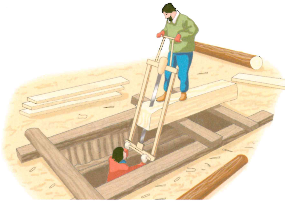
The saw pit
