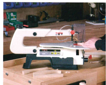
Always keep hands clear of the blade when using the scroll saw
