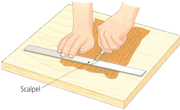
Veneer is cut using a scalpel and a steel rule
