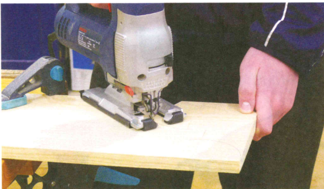
Jigsaw cutting a curve (safety cover removed for clarity)
