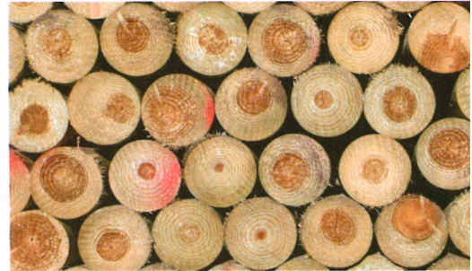
The fence posts have been pressure treated with preservative
