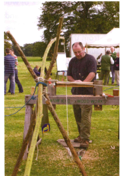
A pole lathe
