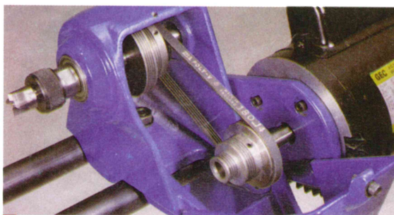
Lathe drive belt
